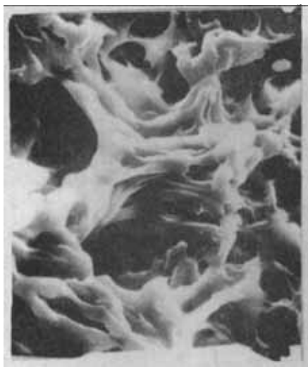
Fig. 3 SEM photograph of poly(NTMAAM-g-AAM) ( \times 418 ) G: 20.5%
